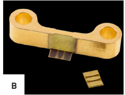
X-MWanchor shown with two GSG jumpers.
